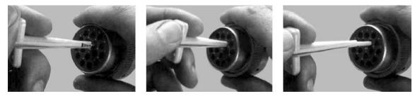
Figure 3-16. HD/HDP Contact Removal
